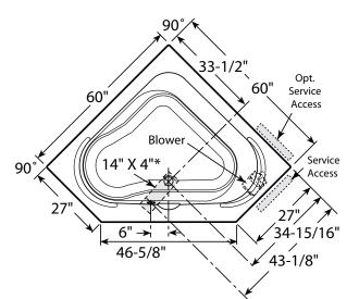
Product Shown: Capella® 60" Pure Air II™ Bath Right Hand Shown Model: BE60 \* Measurements inside unit represent cutout in floor to allow for drain/overflow. Minimum Service Access dimensions given.
